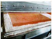
Heated to 820°C, red-hot glass is slumped onto the moulds.
